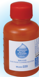
Cleaning Solution 220 (Part no. 3014028653) - contains 10% thiourea and 1% hydrochloric acid (HCl) for removing inorganic residues on sensing membrane and junction
